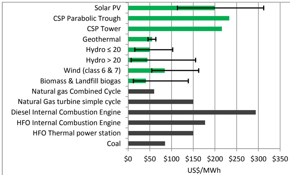
NRET LCOE data from a database by IRENA<sup>55</sup> based on actual LAC project data, excluding Government incentives and subsidies. Green bars show the median values, and error bars show minimum and maximum values. Data for the two CSP technologies, as well as for fossil fuel technologies, are based on a study by IMCO,<sup>56</sup> using fuel price data from Mexico's public utility CFE. Hydro ≤ 20 refers to hydropower under 20 MW.
