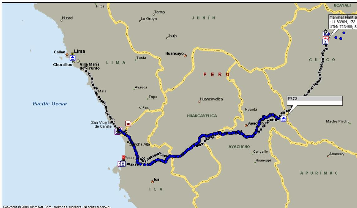
Several routes have been evaluated for the PLNG pipeline. The selected route has been fully surveyed and runs parallel to the TGP gas pipeline, from km 211 to the Pisco area and along the coast to Pampa Melchorita.
